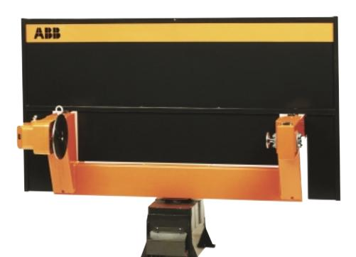
This positioner is for applications requiring two stations – loading and welding – and where the work-piece has to be rotated about one axis.
