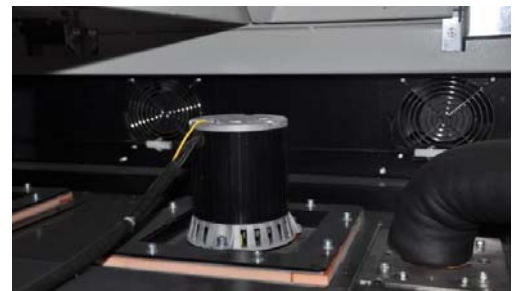
Hot air motor-Blower
